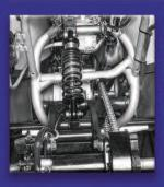
DRR USA engineered this extended square tube swing arm to allow maximum control and traction of the ATV. This provides the rider with a better handling experience.
