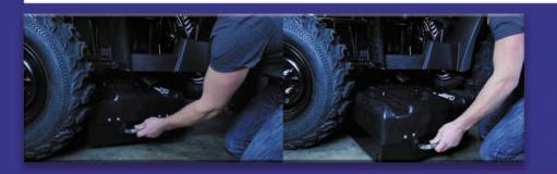
Charge your battery on a standard 120v 20amp outlet or change out the battery for shorter downtime.
