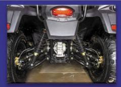
Conquer rough terrains and tough jobs with the ability to switch drives systems with the dual a-arm independent rear suspension. These shocks have five adjustable pre-loaded settings and variable spring rate for optimal performance.
