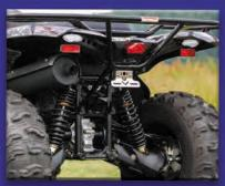
With up to 9 inches of travel, these shocks have five adjustable pre-loaded settings and variable spring rate for optimal performance.
