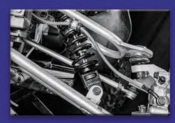
Preloaded adjustable gas shocks with up to 7½ inches of travel for superior performance.
