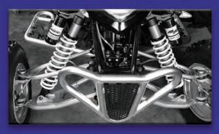
These shocks have adjustable cushioned rebound and preload for optimal performances.
