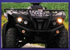
These units come standard with daytime running lights, high beams, and brake lights to signal the rider behind you.
